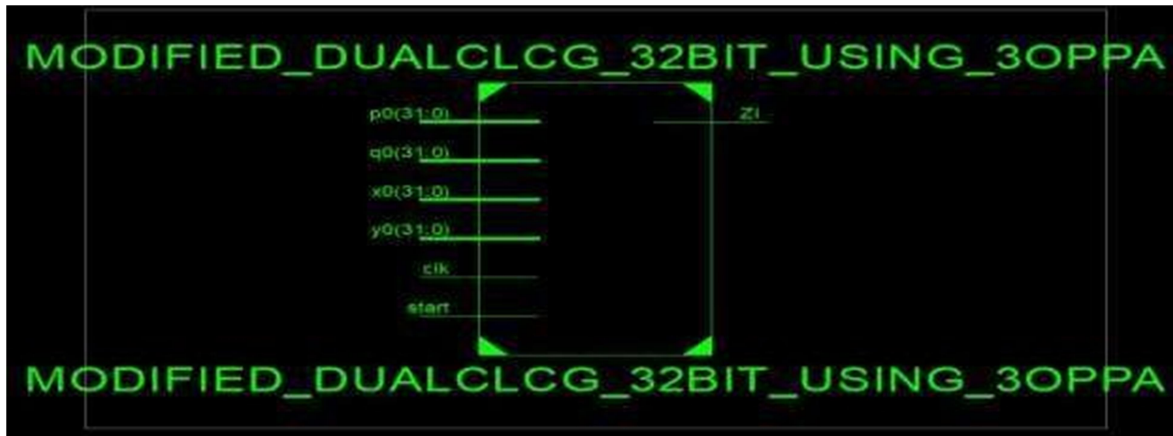
Fig 8.2 RTL Schematic view of proposed Modified Dual CLCG using three operand Adder
