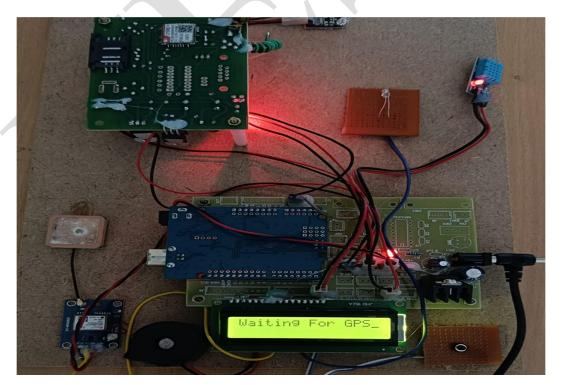
After we have connected the GSM module via a SIM and The System Starts to fetches the current GPS location by providing a message on the LCD as Waiting for GPS as shown in above figure.
