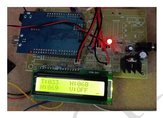
The System counting heartbeat and measuring body temperature correctly. Whenever beat count increase or decrease to certain level or body temperature increases or decreases below certain level system will display the current status of parameters. System also sends the exact location of the soldier when he or she press the panic mode switch to desired Registered Mobile Number through SMS.
