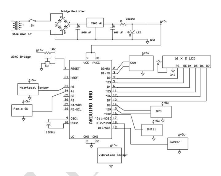
The hardware components are connected to Arduino board. The General purpose I/O pins are connected to buzzer, LCD Display, GSM module, Temperature and humidity sensor, heart beat sensor and GPS modules. 5V RPS is connected to the raspberry pi. The RPS circuit diagram consists of stepdown transformer, bridge rectifier for AC to DC conversion. voltage regulator 7805 for supplying 5V voltage to the Arduino.
