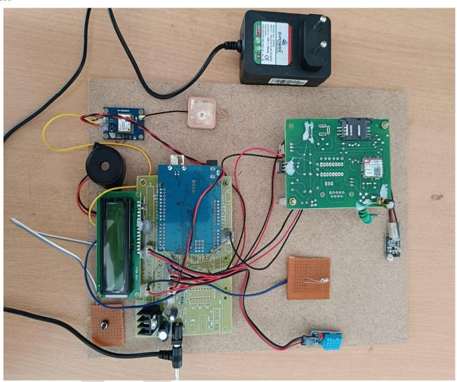
The above image shows the hardware equipment of the project. The kit is turned ON by giving the regulated power supply of 12v which is then converted to 5v dc current. The LED is the indication for 5v current so, if there is 5v current then automatically the LED glows. The generated 5v dc current passes to every hardware co- component in the circuit.
