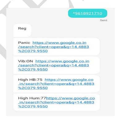
Alert the base unit by alert sound and sends exact location of soldier with the help of GSM and GPS module in the form of text message to desired receiver confirming about GPS geography.
