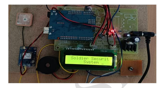
Once the 5v DC current passes throughout circuit the LED is glowed to indicate that the circuit is ready to perform, once the 5v current flows or if we hit the reset button after providing the regulated power supply, the LCD will be displayed the title as SOLIDER SECURITY System. The current output can be seen in the above image.
