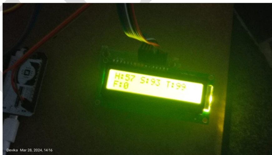
Fig 10: Figure Showing Health Monitoring Data in LCD When Finger Placed on Sensor
