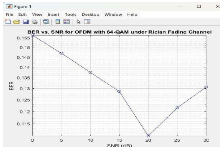
Figure 5.5: BER vs SNR of MIMO-OFDM under Rician(64 QAM)
