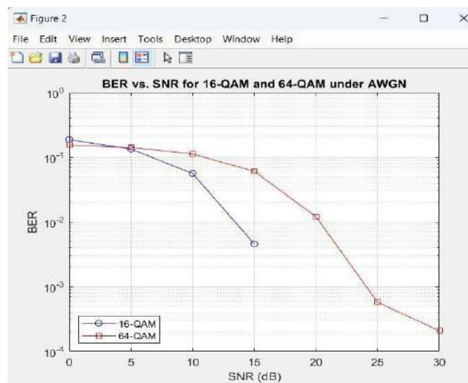
Figure 5.3: BER vs SNR of MIMO-OFDM under AWGN (16 and 64 bit QAM)
