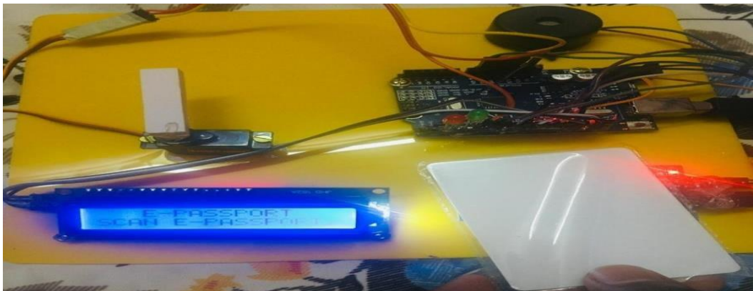
Fig 6.2: If we place an RFID tag near RFID reader it scans and the LCD shows a scan the E-passport
