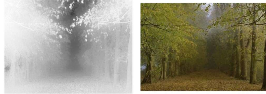
Fig. 6. Atmospheric light estimation and transmission map estimation.
