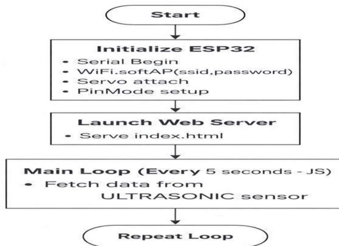
Figure 2; flowchart illustrating the operational sequence of the proposed intrusion detection system using the regulated patrolling robot.
