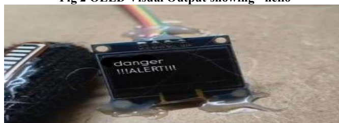
Fig 3 OLED Emergency Alert showing
