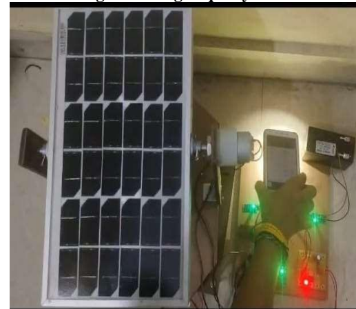
fig 9 Light Falling Equally on All LDRs When equal light intensity falls on all the LDR sensors, their resistances remain nearly the same. Hence, no voltage difference is generated in the
