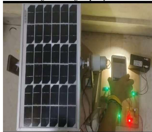
fig 9 Light Falling Equally on All LDRs
