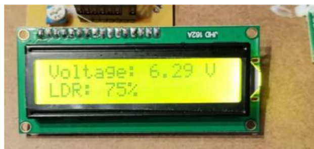
Fig. 7(a) Intensity of the light above 70% (During Day)
