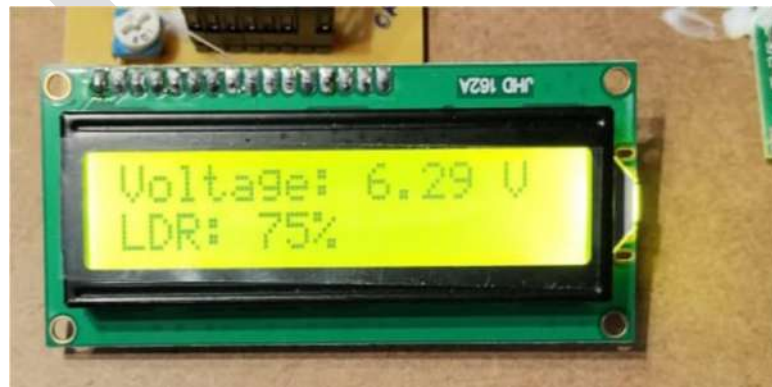
Fig. 5(b) Voltage Generated Under Mechanical Pressure on Piezo Plate
