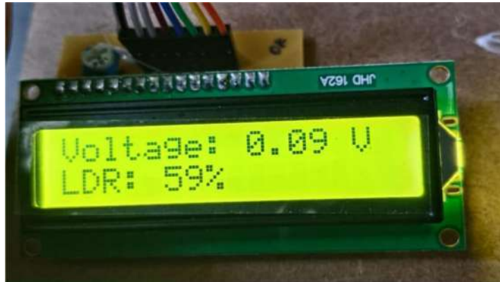
Fig. 4(b) Voltage under no mechanical deformation
