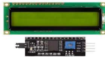
Figure 4 16x2 LCD with I2C Interface
