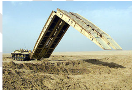
Fig 1.1: M60A1 Armored Vehicle Launched Bridge (AVLB)
