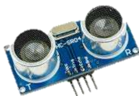
Figure 5: HC-SR04 ULTRASONIC SENSOR
