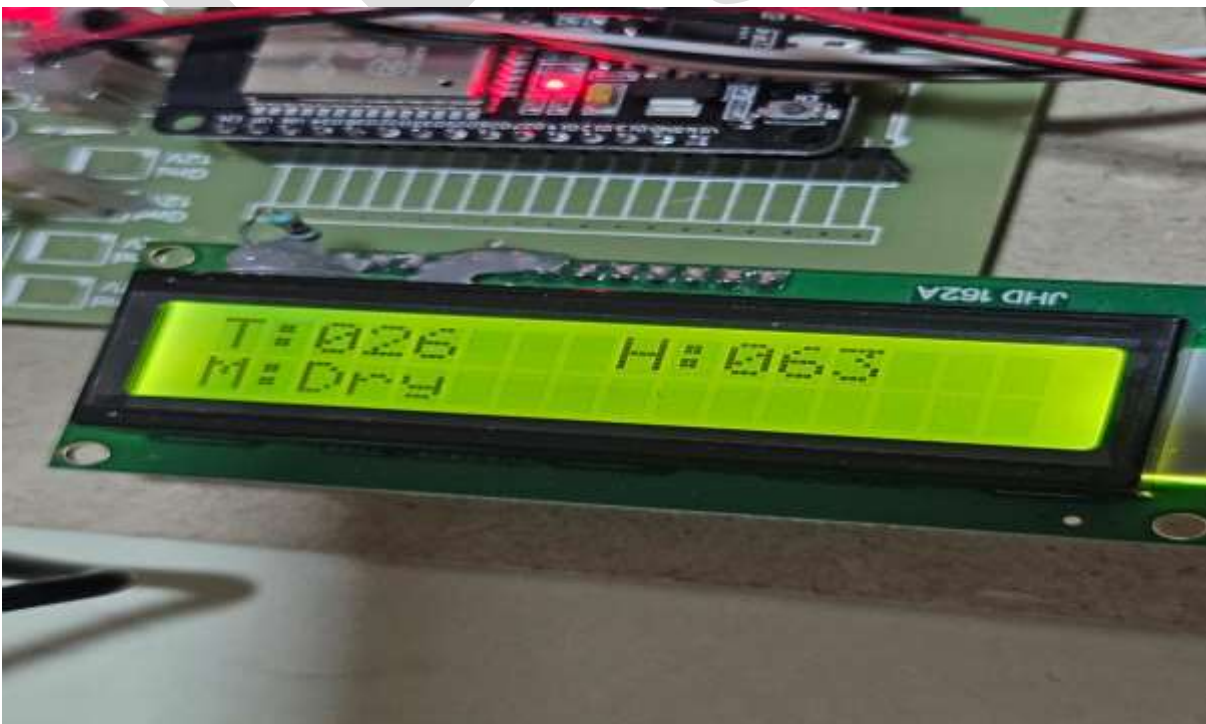
Figure.3: LCD Display the Humidity, Temperature, Moisture
